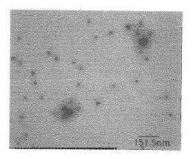
Figure 1 TEM of micelles aerosol-sprayed from a hexanes solution of  $PFP_{50}$ -PDMS<sub>141</sub> (M<sub>n</sub> = 24,000, PDI = 1.14)
